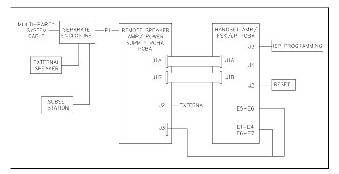
Figure 3. Remote Subset Amplifier Block Diagram
