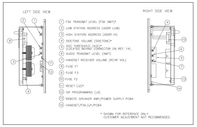
Figure 2. Remote Subset Amplifier Outline Detail
